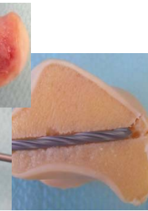
Figure 8 Saw cut through the drilling canal; artificial lesion was hit
